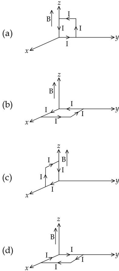
If there is a uniform magnetic field of 0.3 T in the positive  $z$  direction, in which orientations the loop would be in (i) stable equilibrium and (ii) unstable equilibrium ?
